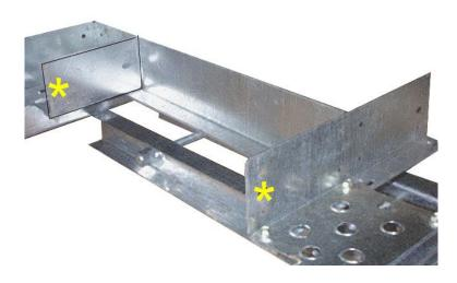
Assemble the  $27^{7/8}$ @x25 ½ " door panel (10). Bolt on the 29" door toe board (11). Using the hardware provided in the hinge kit, bolt on the handle and the hinges. The hinges go on top of the door panel. On the underside of the door panel, use the  $18^{3/4}$  @ hinge stiffener (12). This will be held on with the hinge bolts.
