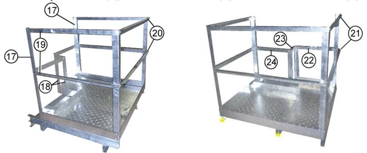
**Note:** At positions noted, bolt on kick braces. Extend them down and fasten the ends to the ladder channels below. This will require drilling a hole in the ladder channels or welding the connection.
