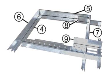
**NOTE:** Using these holes fasten the toe boards to the ladder channels. This will require either drilling holes in the ladder channels or welding the connection.
