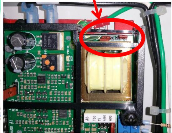
2. To change input voltage to 230VAC move both jumpers to the inside position, as shown below. No other changes are required.
