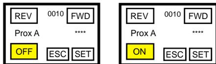
Move the arm to the middle over the home position prox, when this occurs the "OFF" button will switch to "ON"
