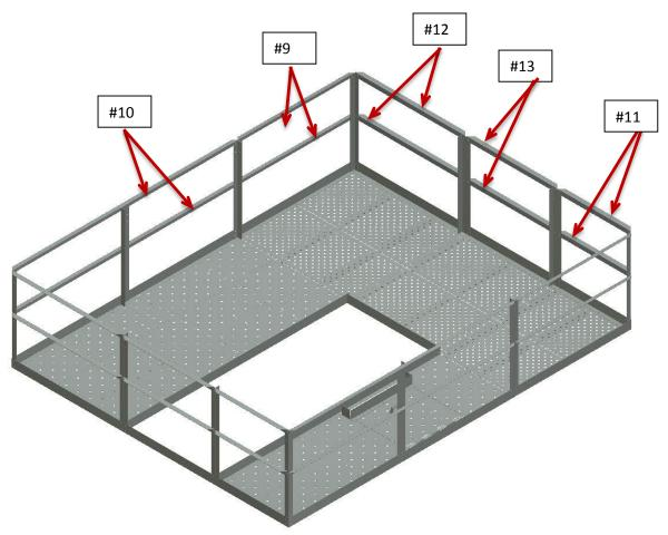
8. Once the floor panels, toe boards, and handrails are all laid out they can be assembled to the secondary support channels using 5/16" bolts. The floor panels can be put on in any order as can the toe boards, but the 1 ½" side of the toe board angle **must go beneath the floor panel** in order to provide the necessary support.
