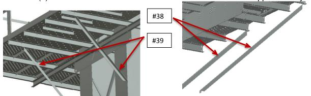
14. The final steps require mounting the head to the trunking. Assemble the handrails and finish bolting the motor mount braces to the motor mount channels on the head. Your platform should now look like the pictures below.
