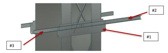
4. Now the **(#3)** rear primary support channels need to be installed. These channels are also 4" deep X 2" wide and are both 77 1/16" long. You will need to elevate the end of the trunk with a boom truck or forklift to install these; also using the 3/8" dia. bolts.
