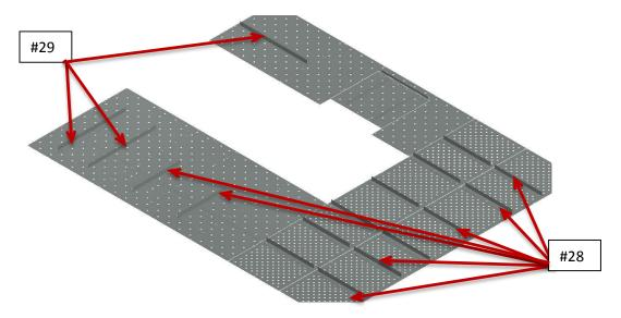
9. Now with the panels all bolted in place and tight, the floor support angles **(#28, #29)** need to be bolted in place using the 5/16" truss bolts. There are (14) of the (#28) 2 x 2 x 26 7/16" support angles and (3) of the (#29) 2 x 2 x 37 9/16" support angles.
