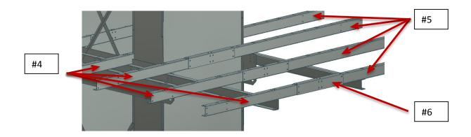
7. To make it easier to install the toe boards (4" X 2" angles) and floor panels, lay them out on the ground as shown in the picture below.
