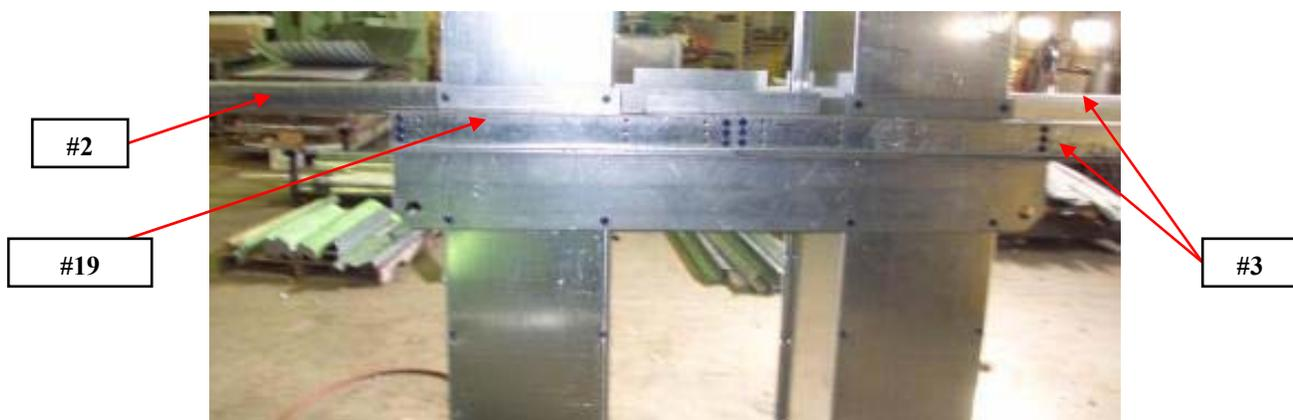
4. Now the (#3) rear primary support channels need to be installed. These channels are also 4" deep X 2" wide and are both  $79 \frac{1}{8}$ " long. You will need to elevate the end of the trunk with a boom truck or forklift to install these; also using the  $\frac{3}{8}$ " dia. bolts.
