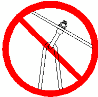
Eyebolt Perpendicular to Rafter ( BAD )
