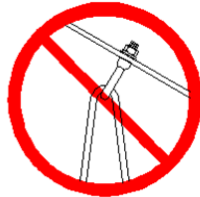
Eyebolt Perpendicular to Rafter (BAD)
