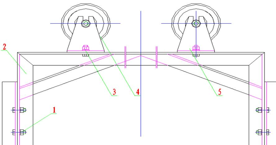
1. Lock nuts 2. Adjustable support 3. Roller lock nuts 4. Support roller 5. Roller support
