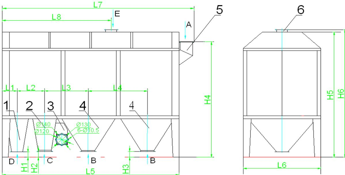
1.Outlet of large impurity 2.Grain Outlet 3.Bottom Air-intake Duct
