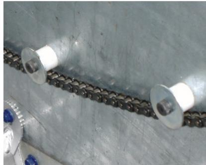
Positive pendulum positioning is achieved through Lambton's high grade roller chain. Precision roller
