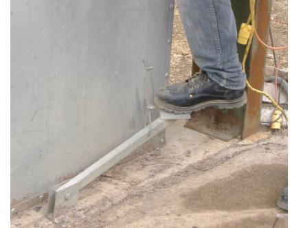
The positive position distributor mechanism is unlatched by using your weight to depress a foot pedal and turning the spout is as easy as turning a steering wheel.
